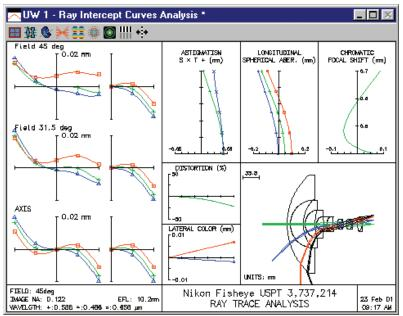
As you can see from the drawing, the aperture stop of the lens is well back in the lens, on surface 14. Obviously the pupil position is a function of the field angle, moving almost to the first surface at the edge of the field. In order to accommodate this type of system and ensure that the rays pass through the desired positions on the aperture stop, OSLO uses the **warm** (wide-angle ray-aiming mode) general operating condition.
