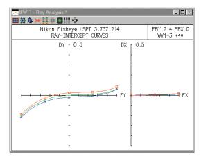
There is some problem in obtaining a graphical field analysis, because all the internal routines extend only to FBY = 1.0. However, the star command \*field accommodates two arguments that give the number of field points and the maximum fby, respectively. The command \*field 12 2.4 produces the following output.
